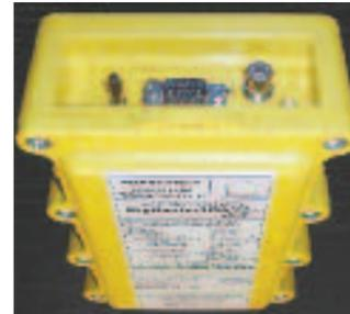
As of 1 February 2009 there is no monitoring by satellites of 121.5 MHz distress signals from Emergency Locator Transmitters (ELTs). Only 406 MHz is monitored by satellites.
